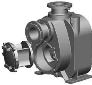
Figure 11: Cleansing of the Casing and the Impeller
